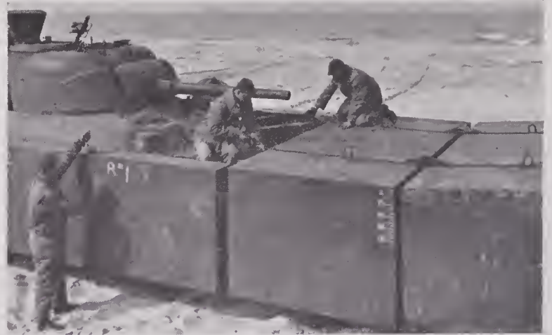
FIGURE 3. Pontons in Ritchie T-6 flotation device are secured with removable pins.
